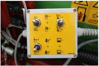
• For all HQ plus models, an electro-hydraulic remote control set for easy operation from the tractor is available as an optional extra
